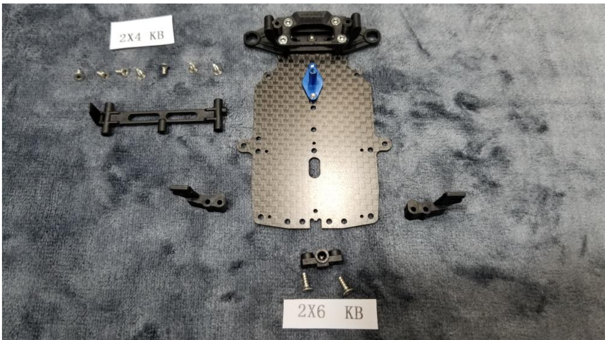
Use the longer 2x6 KB screws to secure the ball link socket
