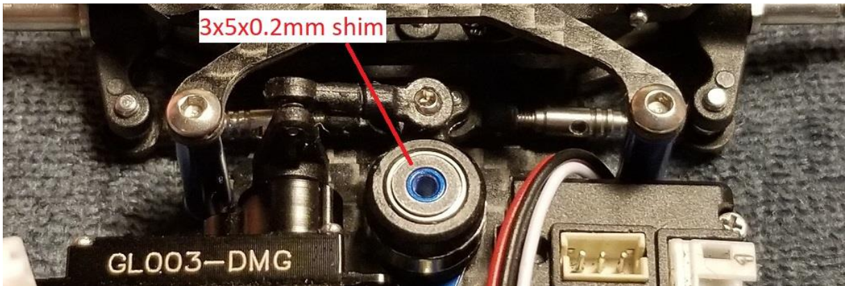
Secure Steering Crank Plate with 2x4 TM and 2x4 KB screws
